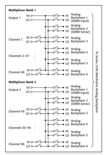
MULTIPLEXER CONFIGURATION: Two independent 1×48 2-pole multiplexers. Banks can be connected together via relays creating a single 1×96 multiplexer. Banks can be isolated from the backplane by relays. Card can be configured for 2- and 4-wire mode.
