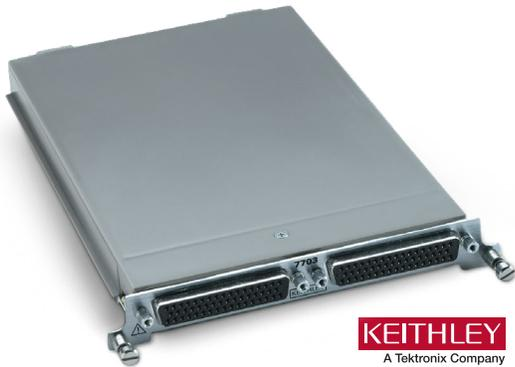
The 7703 plug-in module offers 32 channels of 2-pole or 16 channels of 4-pole multiplexer switching that can be configured as two independent banks of multiplexers. The non-latching reed relays provide high speeds and are designed for 300 volt, 500 mA; 10 VA. The relay closures are stored in onboard memory. The 7703 is ideal for RTD and thermistor temperature applications.
