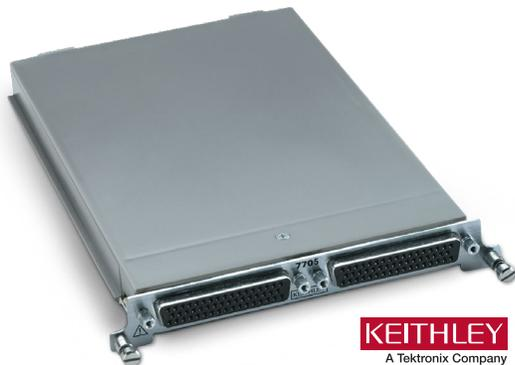
The 7705 plug-in module offers 40 channels of independent switching. These channels are designed to control power to the DUT and switching loads. They can also directly control light indicators, relays, etc.
