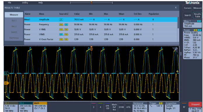
Figure 11. Power Quality Measurements.
