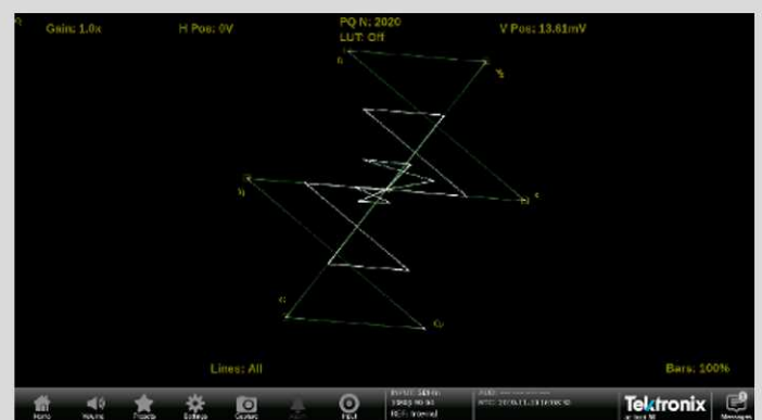
Figure 5: Vectorscope displays – top is for a Rec. 709 and bottom shows the impact of Rec. 2020 (for color bar input).
