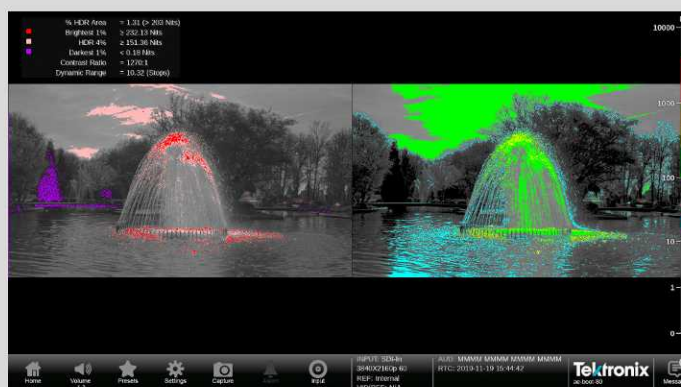
Figure 4: Left display shows lightest and darkest areas in the HDR zone. Right display shows selected key luminance levels in the image.
