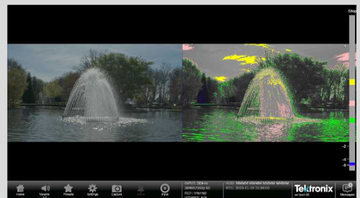
Figure 3: Using banded False Color is an easy way to help set exposure levels.
