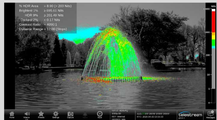
False color display to confirm with standards of brightness, percent HDR and dynamic range of the scene.
