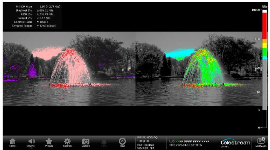
Tektronix display showing false color mode to show out of gamut colors.
