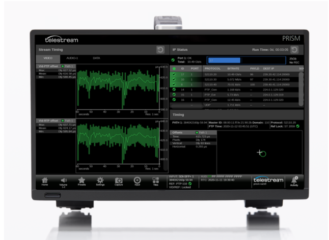
FIGURE 7. PRISM monitoring 2110 streams showing Stream Timing, IP Status and Timing displays.
